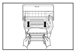
**NOTE:** The *Drum Unit* is sensitive to light. Never expose the *Drum Unit* to light for more than five minutes.
